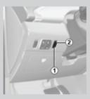
Electric cars are remarkably quiet. This system allows you to warn pedestrians and cyclists. The system is activated automatically when your speed is between 1 and 30 km/h. With the engine running, press the switch (1) to turn the function on or off. The integrated warning light (2) indicates if the function is on or off.
